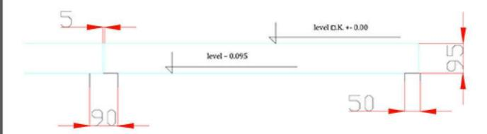
support for two packets - 90 mm peripheral support - 50 mm sub-structure level after providing it with fire protection - 0.095 from O.K.
