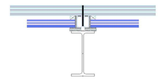
> REI 60 SINGLE CHAMBER GLASS FLOOR BASED ON CONCRETE
