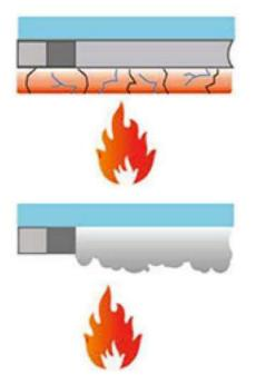
First, fire causes cracking to the external glass unit at stress spots.
